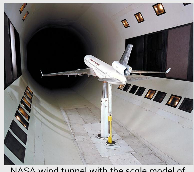
NASA wind tunnel with the scale model of an airplane
